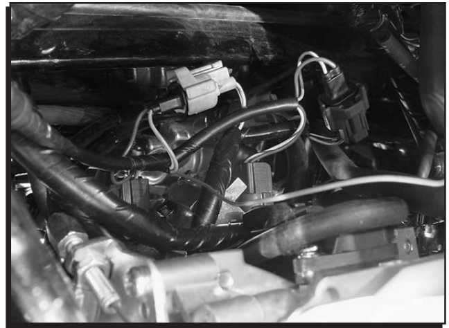
Figure 5 Enhancer Injector Connections.
