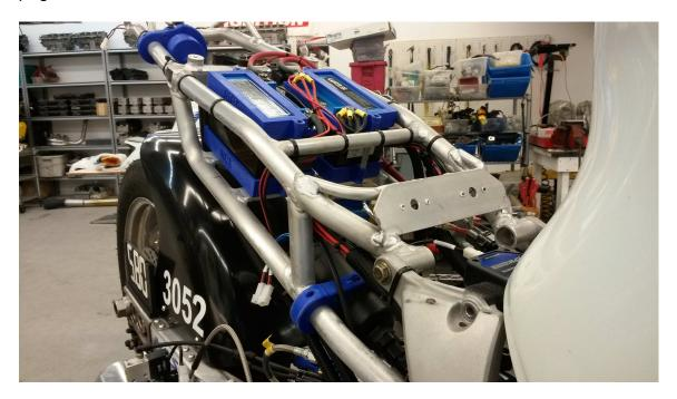
The heart of the bike is of course the "Lethal Injection", a combination of Holley Dominator ecu and MPS Spyder dry nitrous system. It uses MPS 62 lb/hr injectors in stock throttle bodies topped with MPS intake bell and fuel rail. An AEM fuel pump pushes VP C-16 fuel through Earl's hose and Jiffey-Tite quick
