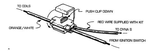
NOTE: The location for obtaining switched 12 volts in Step 11 is one of several possible locations. If a more convenient source of switched 12 volts is available, it may be used, as long as it provides a sound connection. One such source is the 12 volt wire leading to the rear brake stop light switch, and in some cases, unused 12 volt receptacles can be found in the motorcycle's electrical system.
