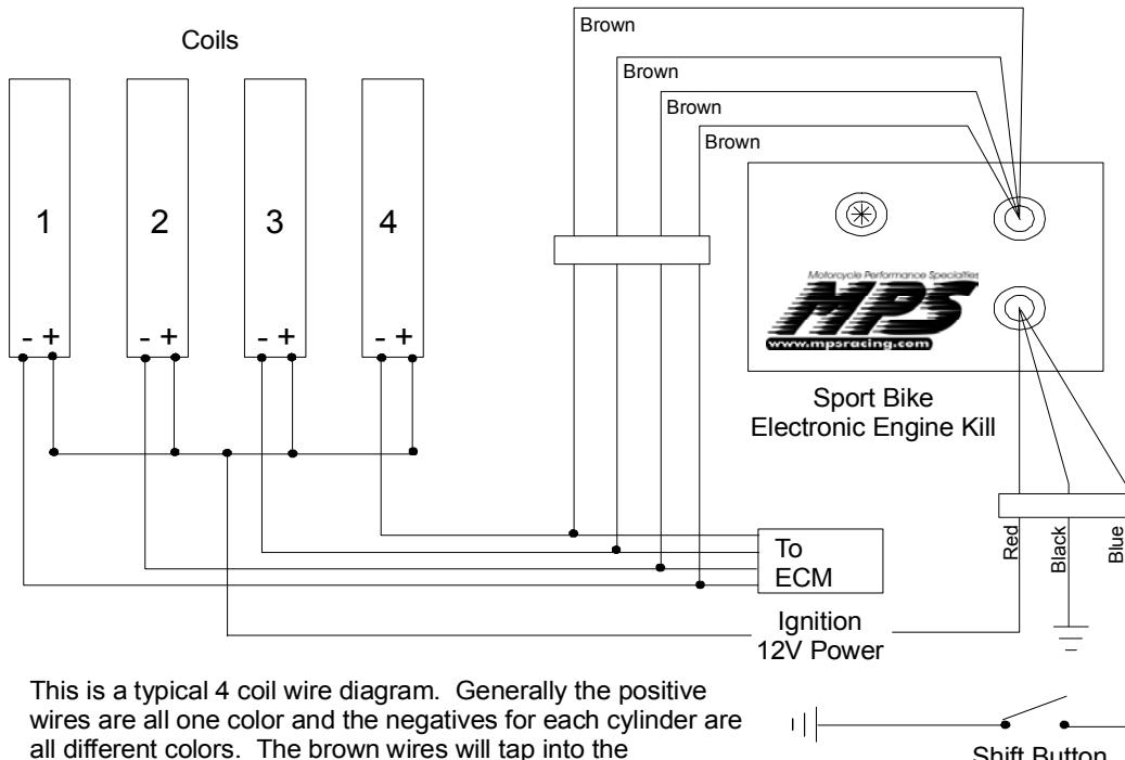
This is a typical 4 coil wire diagram. Generally the positive wires are all one color and the negatives for each cylinder are all different colors. The brown wires will tap into the negatives of each coil.
