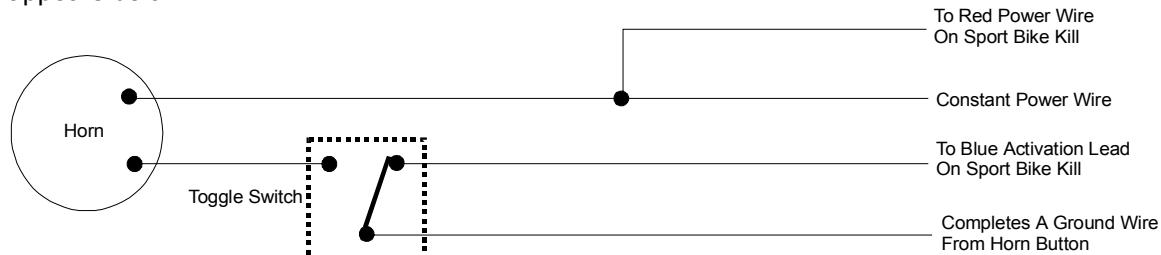
If no wires have continuous power, check them each with the horn button depressed. One of the two should have power with the horn button depressed. This system completes a power circuit to operate. This is the typical Honda and Yamaha horn system. This system requires a SPST relay to be added to the system. A wiring diagram showing how to wire a switch to select the shifter or the horn appears below.
