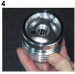
Make sure the three filter element ears are fully engaged in the housing notches. As the filter tightens on the engine the filter element will tighten against the housing which will eliminate any play.
