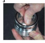
Twist filter element 1/3 turn clockwise (to the right), then let the element spring back up into the locked position.
