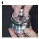
Place the filter element into the housing making sure the three "ears" on the element fall into their slots in the housing.
