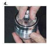
Release the filter element. It should spring up through the 3 slots in the filter housing. You can now remove the filter element for inspection and cleaning
