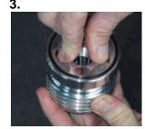
Twist filter element 1/3 turn counter clockwise (to the left)
