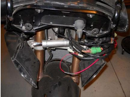
9. With everything connected, you can now test the system. The main battery/charging system will only charge the secondary battery with the key on. Under heavy use with little charging, you may need to charge the secondary battery between rounds (drag racing) but should not need charging under normal use. Ensure that all lose wires are tied and secure before reinstalling the body on the bike.
