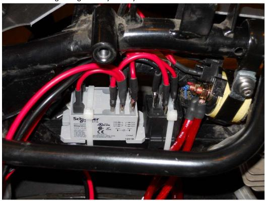
2. On the left side of the tail section, remove the plastic cover that protects the starter solenoid. Disconnect the starter cable from the starter solenoid (lower cable) and the starter. Remove the cable from the bike. Save the black plastic boot that covers the starter nut/bolt. You will re-use it when connecting the new starter cable. Connect the ground cable from the secondary battery to the open (lower) position on the primary starter solenoid.
