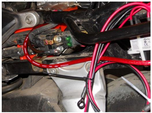
3. The cable labeled starter will route the starter. Make sure it will not be pinched under the tank or along any other moving parts. Using the factory wire restraints under the tank, secure it along the right side of the frame. Connect it using the factory nut/bolt on the starter, using the plastic boot left from the already removed starter cable.
