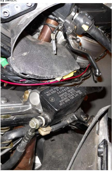
8. Now you will need to connect the Ign. Switch wire to the "Euro" connector located behind the headlight. It will be located on the right side of the headlight harness. It has a factory end on it as to allow for other accessory items to still be utilized.
