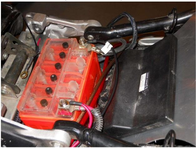
5. Connect the wires label Secondary Battery to the secondary batter located in the tail section. There may be extra wire that will need to be tied up. This is for multiple battery mounting positions.
