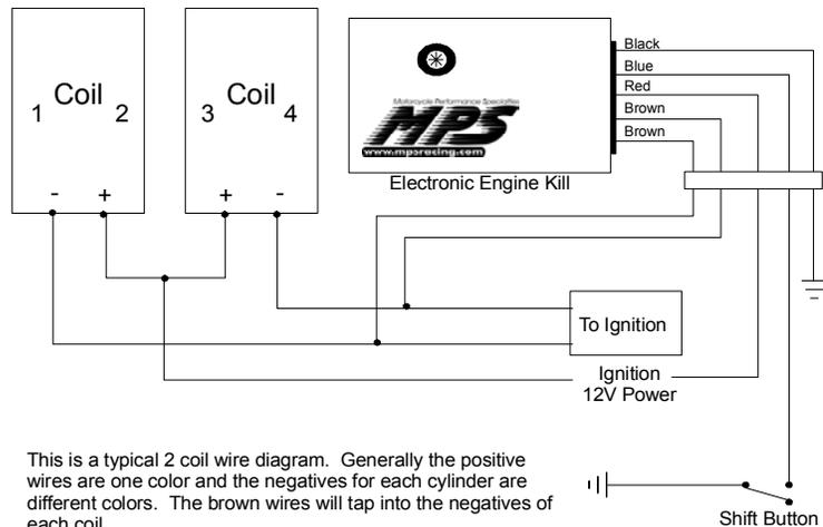
This is a typical 2 coil wire diagram. Generally the positive wires are one color and the negatives for each cylinder are different colors. The brown wires will tap into the negatives of each coil.
