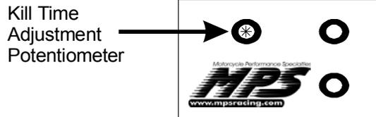
start with to much kill time and work your way quicker. We generally start at around 75 ms. of kill time. The Kill Time is adjusted via a small potentiometer accessed through the grommet on the front of the unit. Using a small screwdriver Carefully turn the pot
