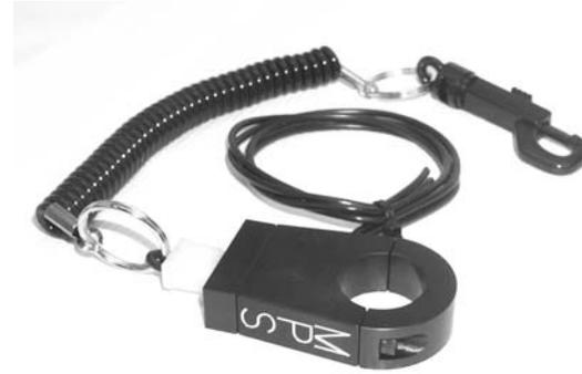
**Installation** – To install your Tether Kill Switch first find 1/2" of open handlebar space. On some bikes you may have to slide switch pods or master cylinders a little to get the room necessary. Take the horseshoe shaped back off the switch and fit the switch onto the handlebars. Replace the back and tighten the mounting screws with the plug facing the rider.
