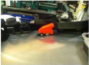
9. Test the system, Part 2. With the switch in the open position, turn the key on. Again, a click should be heard. If not, go back to step 7. Start the bike. The bike should start with the factory original 12v starter. This is only intended as a fail-safe measure in the event that the 24v system does not operate as intended. If the 2<sup>nd</sup> battery is dead or a wire come loose/broken, this will allow you to start the bike.
