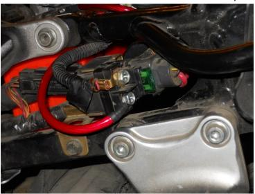
3. The longest 8 gauge wire will connect to the starter. Route the starter cable to the starter. Make sure it will not be pinched under the tank or along any other moving parts. Using the factory wire restraints under the tank, secure the new starter cable along the right side of the frame. Connect it using the factory nut/bolt on the starter, using the plastic boot left from the removed starter cable.
