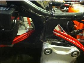
2. On the left side of the tail section, remove the plastic cover that protects the starter solenoid. Disconnect the starter cable from the starter solenoid (lower cable) and the starter. Remove the cable from the bike. Save the black plastic boot that covers the starter nut/bolt. It will be re-used when connecting the new starter cable. Route the shorter 8 gauge cable across the bike behind the battery to the starter solenoid. Connect it to the lower starter solenoid terminal as pictured.
