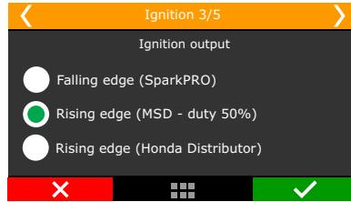
**Falling edge (SparkPRO):** Select this option when using FuelTech SparkPRO, M&W ignition, smart coils (integrated igniter, such as GM LS coils). This mode has dwell control enabled. It's important to know the dwell requirements or “charge time” of your particular ignition coil(s).
