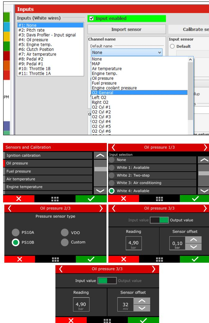
The FT600 has fully customizable inputs, which allows to read any 0-5V analog pressure sensor, since its pressure vs voltage table is known. In this case, just select the custom option and fill the interpolation table through FTManager.
