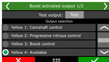
Select an available output to trigger a relay or any other external device.
