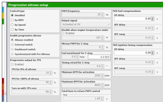
Select an auxiliary output as "Progressive nitrous output" and how the control will be performed: by time (after 2-step), by rpm or by wheel speed.
