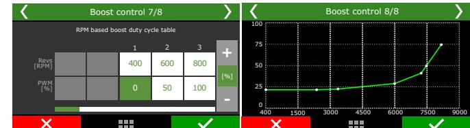
At last, there will be the boost duty cycle table by rpm, speed or time. The boost by time starts after the 2-step release.
