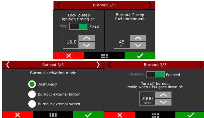
But when the two-step button is being pressed, the value considered is the one set for the two-step parameter. The values adopted for ignition timing retard and enrichment are the ones configured on the two-step function.
