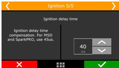
That's the delay time the ignition module has between receiving a signal to spark and effectively spark at the plugs.
