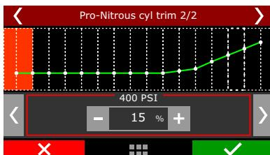
**Nitrous stage timing tables:** After the delay, there are the timing tables to each stage. You can program the timing compensation over RPM and it is calculated considering the main timing table. In the FTManager software is possible to visualize the total calculated ignition table.
