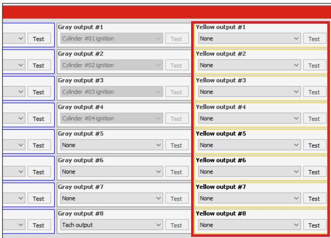
Select the outputs that will control the two wires from the throttle motor. By standard they are yellow #3 (motor 1A) and yellow #4 (motor 1B). In case these outputs are already being used by another kind of control, use outputs yellow #1 and yellow #2
