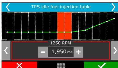
This menu is only available when the idle speed is set up by TPS. The injection time is adjusted according to the engine RPM.
