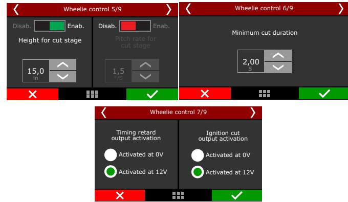
As the retard stage, the cut stage also has height and pitch rate settings. Since it is a safety measure, the ignition cut level is 90%.
