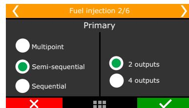
**Sequential:** in this mode, each injector output fires only a single time per engine cycle (720° on a 4 stroke). This mode is only available when a cam sync sensor is properly set up.
