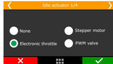
An important tip is that, when selecting "No Actuator", it is still possible to control idle speed by ignition timing as configured in the "Other Functions" then "Idle Speed" menus. If any kind
