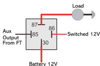
The auxiliary outputs must be set manually according to the desired function in the outputs (blue, gray or yellow wires) that are not being used as injector or ignition outputs.
