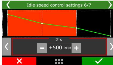
**Compensation by load:** used to compensate actuator position when suddenly loads (like AC or fan) are added to engine and can affect idle. It is possible to set an target RPM compensation when the AC is on and fuel/actuator opening compensation for AC and fans.
