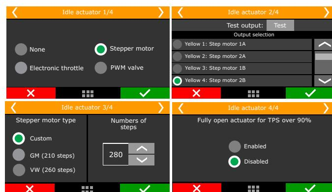
The option "Fully open for TPS over 90%" fully opens the idle valve when TPS is above 90%, increasing the air admitted.
