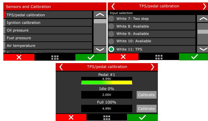
TPS sensor must be calibrated on the first time the ECU is turned on only, and should be recalibrated only when it has to be replaced or the throttle opening on idle was changed. TPS calibrations are individual by map file.
