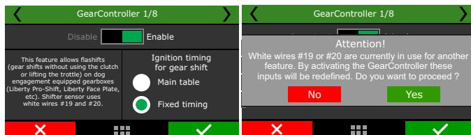
**Cut duration:** the cut duration configuration is adjusted in ms and the values are configurable by gear.
