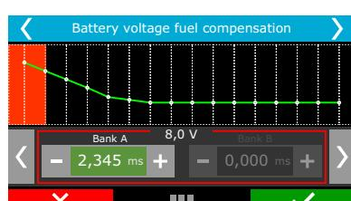
With lower battery voltages the injectors takes a longer time to open and to close. This table is used to compensate this variation.
