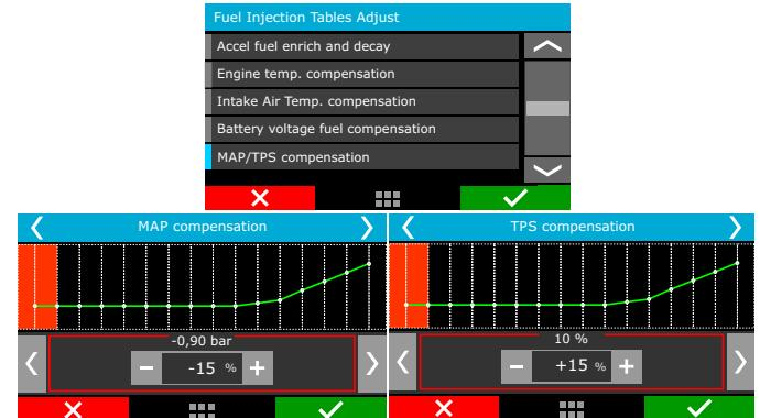
This table changes according to the main map configuration (MAP or TPS). When the main fuel table is setup by MAP, this table is a compensation by TPS. When the main fuel table is setup by TPS, this compensation is by MAP.
