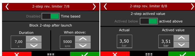
To prevent the driver to activate the 2-step on a run, there are 2 safety parameters. Block 2-step by time or by RPM. This way, even if the driver press the 2-step button, it will not activate before the time slip or above the RPM.
