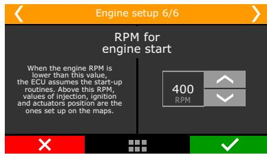
**RPM for engine start:** set up a RPM limit above which the start-up routines are disabled. Below this RPM, all the injection, ignition and actuator positions set up for engine start are used.
