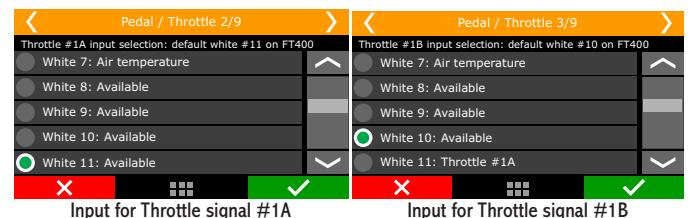
Now, setup the inputs that will be connected pedal #1 and pedal #2 position sensors. The standard inputs are wires white #9 (pedal #1) and white #8 (pedal #2).
