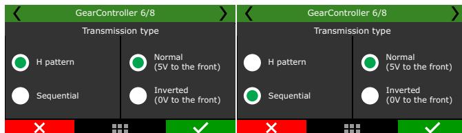
With the car stopped, push the shifter to the front and check the voltage read in the FT600 diagnostic panel. The recommended value is between 4 and 4.5V (or 0.5 and 1V - inverted transmission).
