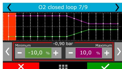
O2 closed loop control limits is a 16 points (8 columns and 2 lines) table, totally editable, by TPS or MAP, which defines the actuation limits of O2 closed loop, avoiding the control to remove or add too much fuel in certain situations.
