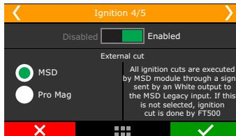
This mode is only available when using a distributor and a MSD ignition module. Enabling this option means the ignition cuts will be performed by the MSD using the Legacy input they have.
