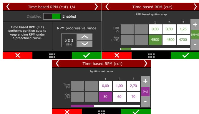
It will perform ignition cut to keep the wheel speed/driveshaft RPM under a predefined curve.
