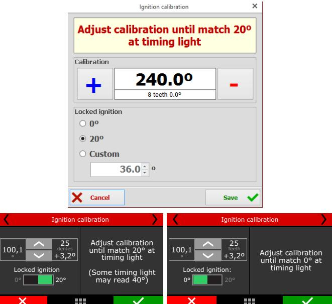
**Ignition calibration with crank trigger:** Cars originally equipped with crank triggers, usually do not have the TDC mark. This mark then should be done by stopping the engine on cylinder #1 TDC of compression using a dial-comparator. It is very important to be precise when making this timing mark; the slightest error will ultimately affect ignition timing on the engine
