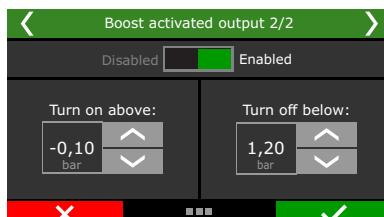
Select the output signal sent when it is activated. The only outputs capable of switch 12V are the yellow.
