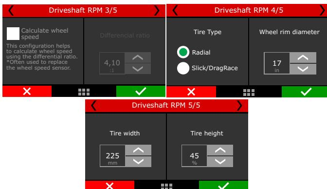
To calculate wheel speed, insert the differential ratio and tire dimensions.
