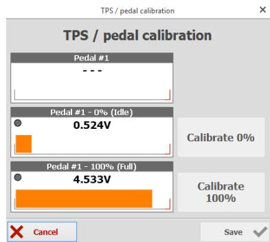
**Possibly disconnected:** check TPS connections. Maybe there is a broken wire or one of the connectors does not reach the TPS pins. Check with a tester to see if the voltage on the orange wire varies according to the throttle position.
