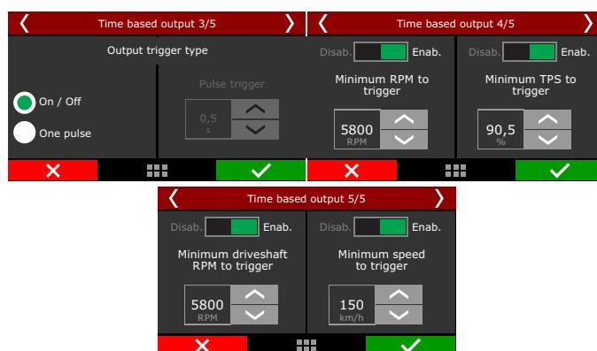
All this options can be enabled or disabled. The output signal can be an ON/OFF signal (remaining on while the conditions are valid) or a pulse (to release the parachute, for instance), which the duration is programmable
