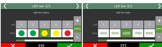
**By gear:** select the LED to edit, choose its color, set the RPM you want it to turn on for each gear and which LEDs will be activated.
