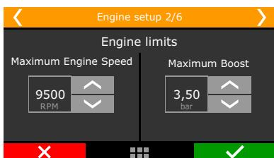
**Maximum engine speed:** setup the engine maximum RPM. All fuel and timing maps will be created with its last point on this RPM. This parameter is also used to calculate fuel injector's percentage of use.
