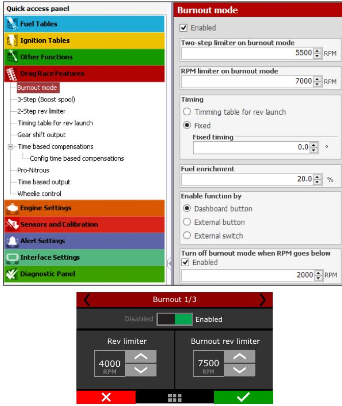
When Burnout mode is activated, it disables the standard RPM Limiter, instead the ECU uses this RPM limiter as the engine's RPM limit.
