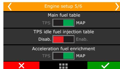
**MAP:** this mode is indicated for turbo or naturally aspirated engines. That's the mode that better represents engine load, because engine vacuum varies under different loads, even with the throttle on the same position.
