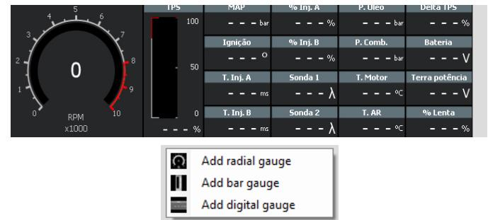
To add or remove gauges, click with mouse right button in a free space and select the gauge type you want to (radial, bar or digital).
