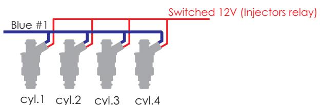
Even with each output controlling only one injector it is possible to change the triggering mode to multipoint (batch fire), semi sequential (outputs triggered in pairs) or sequential.
