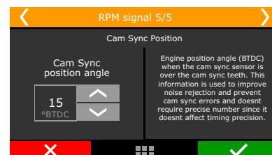
This angle is not mandatory and won't affect the ignition calibration. If you don't know the position angle, set the same alignment as crank index position or select the cam sync sensor as random.
