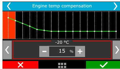
This compensation is applied based on the engine temperature sensor, which, in water-cooled cars, must be at the cylinder head reading the water temperature, and in air-cooled engines, must be reading the oil temperature.
