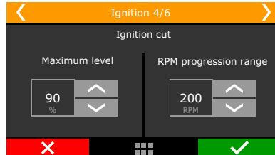
The ignition cut maximum level is the percentage of ignition events that will be cut to limit the engine RPM.
