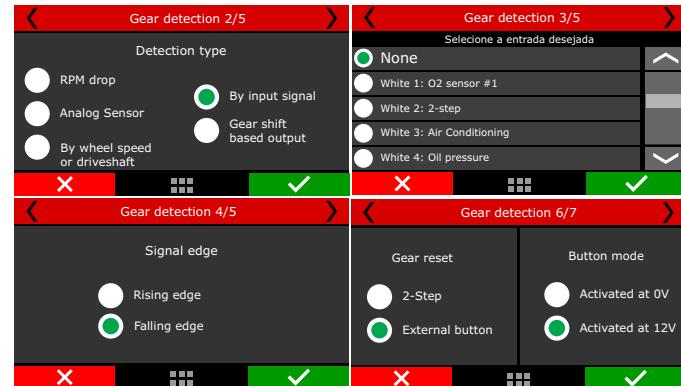
The fifth mode enables an internal counter that is increased by each pulse sent out by the Gear shift output (Drag Race Features menu). This mode cannot detect downshifts and requires the 2-step to be used to reset the counter; therefore it is best suited for drag race cars.
