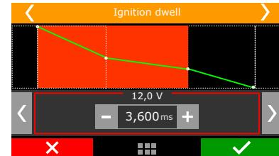
This option sets the ignition coil charging time. There is a dwell table because the charging time varies according to the battery voltage, especially in vehicles that do not have alternator.
