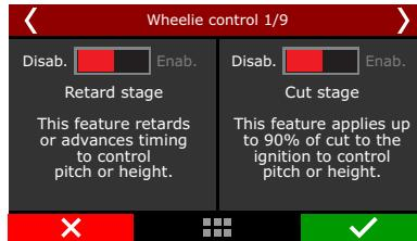
The retard stage always retards timing when the vehicle's front end exceeds a predefined height. The ignition cut stage cuts the ignition to control the front end height.
