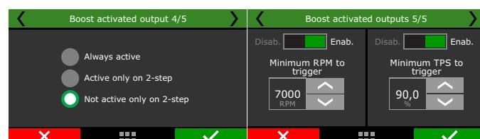
There are 3 different activation modes: "always active", "active only on 2-step" or "Not active only on 2-step". This means that even if the vacuum/boost conditions are met, the activation mode condition must be respected.
