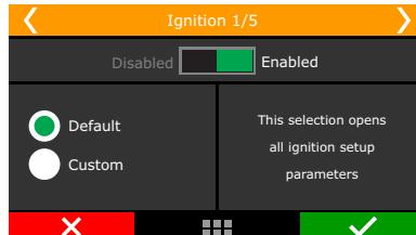
**Default:** this mode makes available the options that are commonly used for the majority of engines, with standard firing order tables and configurations.
