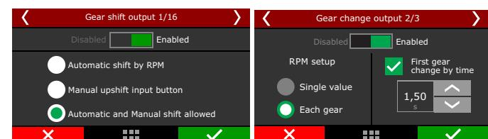
Select the desired output, all the outputs will be displayed, except the ones used for injection and ignition. In the FTManager, this setup is at "Sensors and calibration" - "Inputs".
