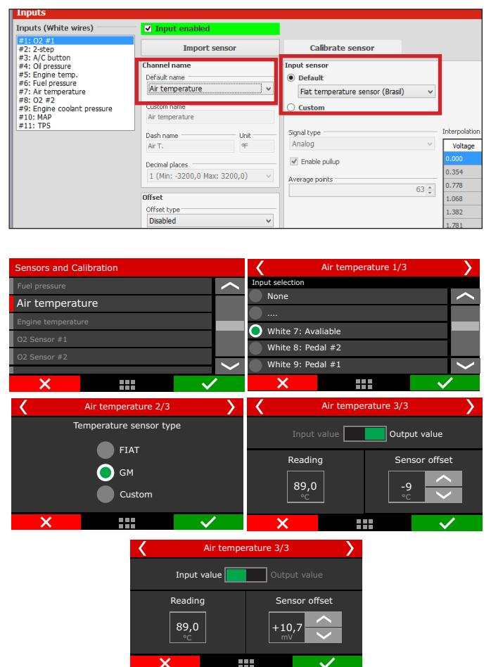
The FT600 has fully customizable inputs, which allows to read any 0-5V analog temperature sensor, since its temperature vs voltage table is known. In this case, just select the custom option and fill the interpolation table through FTManager.
