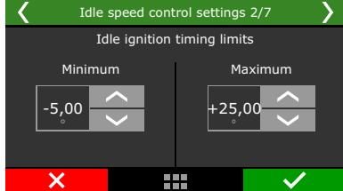
This control uses a target RPM for idle speed and works advancing and retarding the engine timing to keep the engine running near the specified RPM.
