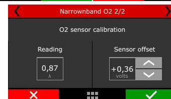
4. If the calibration and configuration are correct, there will be no reading difference.
