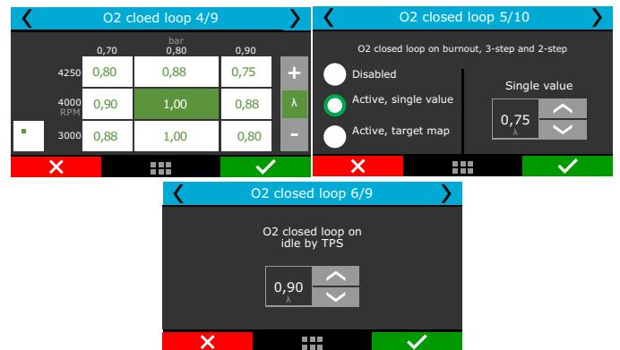
Next, is a 3D table of O2 closed loop targets versus RPM and MAP. It has up to 16x16 cells that can be edited through the PC Software.
