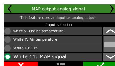
The MAP signal can be read in an external datalogger.
