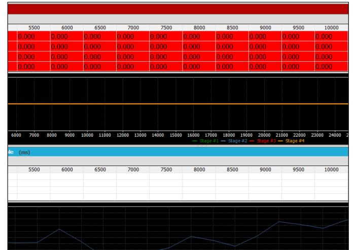
On the first screen is the configuration that allows setting a delay to start the fuel compensation, based on the time that the nitrous shot takes to get to the combustion chamber.
