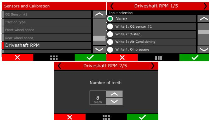
With the driveshaft speed and the tire dimensions, it is possible to calculate the traction wheel speed. If you want to use a driveshaft RPM sensor instead of a wheel speed sensor, check the box "Calculate wheel speed" in the next screen.
