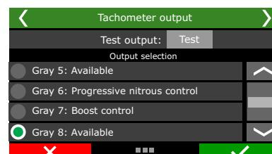
If one of this outputs are not available, the blue #1 to #8 and grey #1 to #7 can also be used, but an external 12V pull-up with a 1K resistor.
