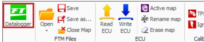
open the FTManager, and click on the Datalogger icon. The FTManager Datalogger will open. To download, click on the Download icon and a window will pop up showing all logs saved on the ECU. Select the files and click ok.
