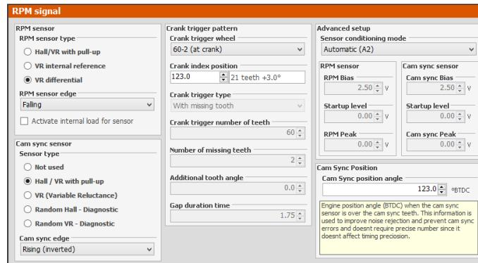
**Engines with crank trigger:** select the crank trigger pattern.
