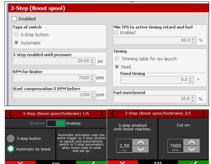
There are two ways to activate this function, one uses an external button (must use a white wire attached to a button, usually on the foot brake) and the other is through 2-step button.
