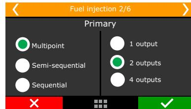
**Semi-sequential:** in this mode, injectors are fired once per engine revolution, at 0° and 360°, in pairs, according to the twin cylinders. In a 4 cylinder engine, cylinders 1 and 4 will be fired at the same time, then cylinders 2 and 3 at the same time.
