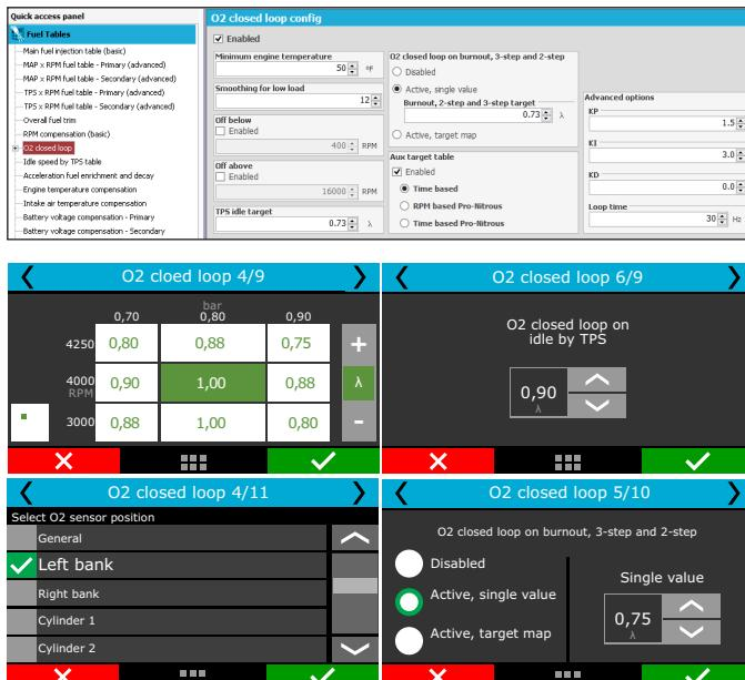
Low load smoothness is the speed control for low load situations like idle speed, where the O2 closed loop must reduce the compensation for O2 variations.
