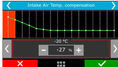
This compensation is applied based on the air temperature sensor placed in the intake manifold, and it is only available when the sensor is connected to the injection system.
