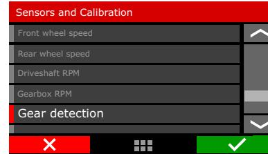
In this menu there are the settings related to gear detection change (display and log). There are 5 different ways to detect it: by RPM drop (drag race only), by gear position sensor (requires a sensor in the transmission), by interpolating the current wheel speed versus engine RPM, by pulse and by gear shift output.
