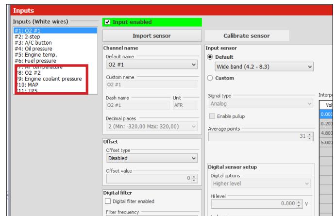
After inserting the Throttle code, set the input that will be connected to the throttle position sensor, usually there are two signals on the throttle. Standard inputs are wires white #11 (Throttle signal #1A) and white #10 (Throttle signal #1B).
