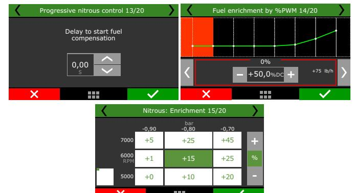
The ON delay for NOS fuel compensation avoids the extra fuel to get earlier than the NOS in the cylinder, very common when the fogger is far from the injectors.
