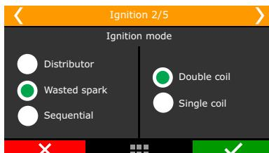
The option “distributor” means that the spark distribution will actually be done by a distributor, with a single coil, regardless of the number of cylinders. Only the ignition output #1 (gray #1) will be used to control the ignition coil, the others are disabled.
