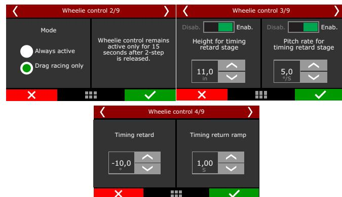
You can set as always active or drag racing mode. In drag racing mode, the control will work for only 15s after 2-step.
