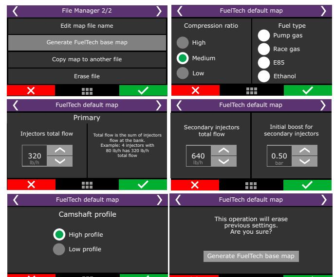
**Compression ratio:** used to correctly estimate the timing tables. A low, medium or high compression ratio is defined according to the fuel used on the engine and if it is turbocharged or naturally aspirated. I.e., a 10:1 compression ratio for a naturally aspirated engine using ethanol is considered a "low compression ratio". The same ratio for a turbocharged engine running gasoline will be "high".
