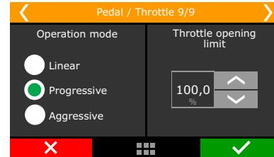
The last parameter to be configured is an opening limiter, very useful to limit the engine power by the throttle.
