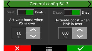
**Proportional output:** from 10% TPS the output is proportional to the map. The programmed pressure is reached when the TPS reaches the value set.
