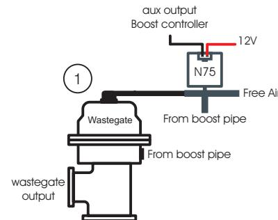
Example 2: the second way is to connect the boost solenoid to the top of wastegate.
