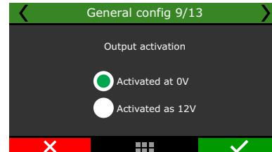
Set the solenoid trigger output
